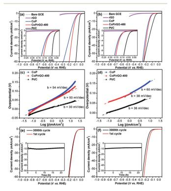
Fig. 2 Electrochemical HER activity of CoP/rGO-400. (a) LSV curves, (c) Tafel slopes and (e) durability test in 0.5 M  $\rm H_2SO_4$  solution; (b) LSV curves, (d) Tafel slopes and (f) durability test in 1 M KOH solution. Insets in (e and f): time-dependent current density curves under static overpotentials of 105 mV in 0.5 M  $\rm H_2SO_4$  and 150 mV in 1 M KOH solution, respectively.
