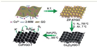
$\begin{tabular}{ll} {\bf Scheme 1} & {\bf Illustration of the fabrication procedure for the CoP/rGO-T nanocomposite.} \end{tabular}$
