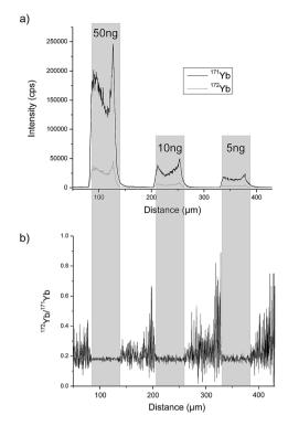
Fig. 2 LA-ICP-MS analysis of gel electrophoresis spots containing 50 ng, 10 ng and 5 ng of MeCAT(Yb)-IA labeled HSA spiked with isotopically enriched MeCAT( $^{71}$ Yb)-IA labeled HSA in a proportion 1 : 2: (a) signal intensities of isotopes  $^{171}$ Yb and  $^{172}$ Yb. (b) Isotope ratio  $^{172}$ Yb/ $^{171}$ Yb (reproduced from ref. 8 with permission from the Royal Society of Chemistry).
