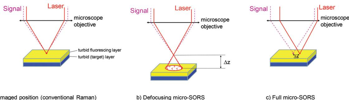
**Fig. 1** Schematic diagram of (a) conventional Raman microscopy of the turbid stratified sample (‘imaged’ position), (b) defocusing micro-SORS and (c) full micro-SORS in a situation with a highly fluorescing overlayer followed by a target layer from which the Raman signal is desired (Raman signal – dashed line, laser beam – solid line).
