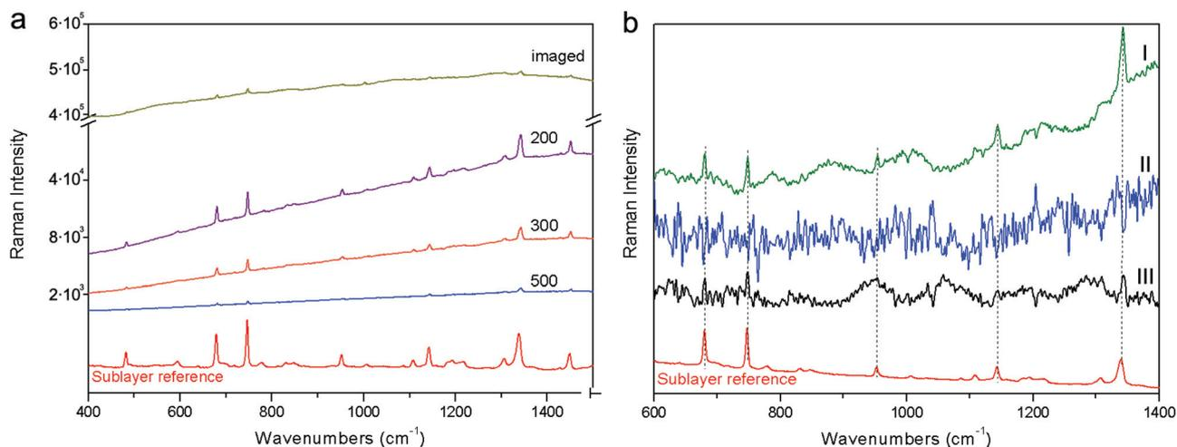
**Fig. 5** S3: full micro-SORS (a) sequences. Spatial offsets in  $\mu\text{m}$  are indicated next to the spectra. Subtraction results (b); full micro-SORS subtraction between 'imaged' and 200  $\mu\text{m}$  offset (I), defocusing subtraction between imaged and 1000  $\mu\text{m}$  defocusing distance (II) and conventional Raman imaged baseline subtracted (III). Reference spectra are shown in red.
