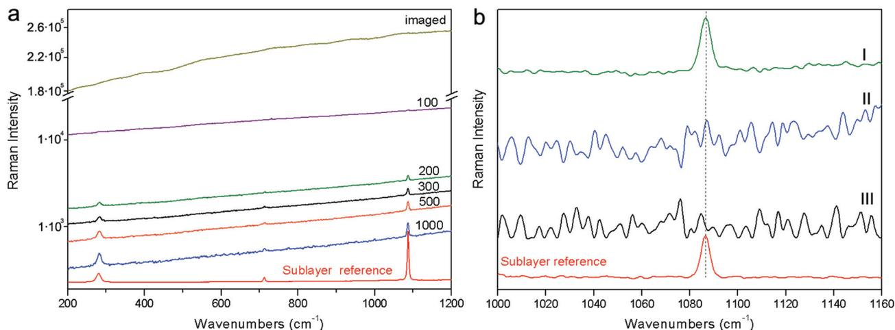
**Fig. 6** S4: full micro-SORS (a) sequences. Spatial offsets in  $\mu\text{m}$  are indicated next to the spectra. The spectra are plotted on a logarithmic scale. Subtraction results (b); full micro-SORS subtraction between 'imaged' and 1000  $\mu\text{m}$  offset (I), defocusing subtraction between imaged and 1000  $\mu\text{m}$  defocusing distance (II) and conventional Raman imaged baseline subtracted (III). Reference spectra are shown in red.
