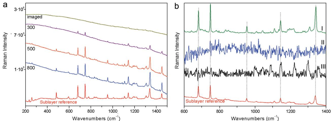
**Fig. 4** S2: full micro-SORS (a) sequences. Spatial offsets in  $\mu\text{m}$  are indicated next to the spectra. The spectra are plotted on a logarithmic scale. Subtraction results (b); full micro-SORS subtraction between 'imaged' and 800  $\mu\text{m}$  offset (I), defocusing subtraction between imaged and 1000  $\mu\text{m}$  defocusing distance (II) and conventional Raman imaged baseline subtracted (III). Reference spectra are shown in red.
