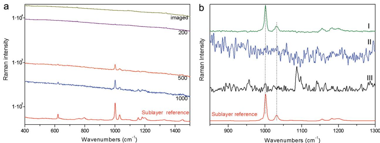
**Fig. 3** S1: full micro-SORS (a) sequences. Spatial offsets in  $\mu\text{m}$  are indicated next to the spectra. The spectra are plotted on a logarithmic scale. Subtraction results (b); full micro-SORS subtraction between ‘imaged’ and 1000  $\mu\text{m}$  offset (I), defocusing subtraction between imaged and 1000  $\mu\text{m}$  defocusing distance (II) and conventional Raman imaged baseline subtracted (III). Reference spectra are shown in red.
