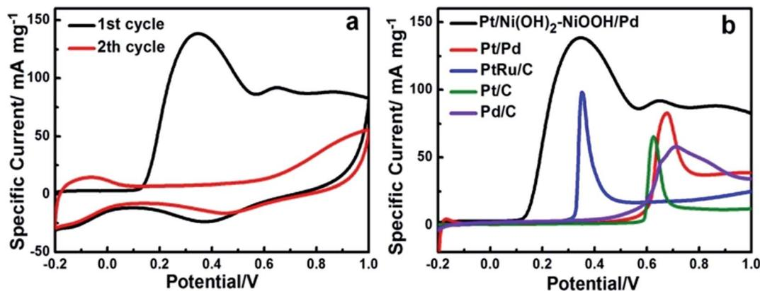
Fig. 4 (a) CO stripping voltammograms on the Pt/Ni(OH)<sub>2</sub>-NiOOH/Pd MHNRRs performed in a solution of 0.5 M H<sub>2</sub>SO<sub>4</sub> at 20 mV s<sup>-1</sup>; (b) the comparison of the CO stripping voltammograms of the Pt/Ni(OH)<sub>2</sub>-NiOOH/Pd MHNRRs, Pt/Pd MHNRRs, commercial Pt/C, Pd/C and PtRu/C catalysts.
