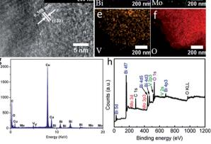
Fig. 3 (a) The HETEM image, (b) HAADF-STEM image, elemental mapping images of (c) Bi, (d) Mo, (e) V and (f) O, (g) EDX spectrum and (h) the survey XPS spectrum of  $BiMo_{0.015}V_{0.985}O_4$ .
