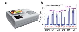
Fig. 6 (a) Photograph of the integrated PEC platform. (b) Photocurrent responses of the  $BiMo_{0.015}V_{0.985}O_4$  modified ITO electrode in the integrated PEC platform without (blank PBS solution) and with the addition of a certain volume of juice to 4 mL of 0.1 mol  $L^{-1}$  PBS (pH = 7.4).
