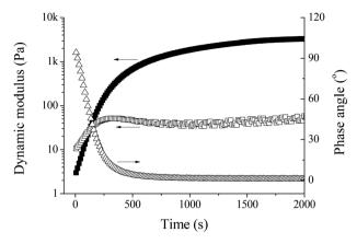
Fig. 3 Evolution of the storage modulus  $G'(\blacksquare)$ , loss modulus  $G'(\square)$  and phase angle  $\delta(\triangle)$  of a 4.0 wt% Alg–DA solution (DS = 21%) with time in the presence of HRP (23.04 U mL<sup>-1</sup>) and H<sub>2</sub>O<sub>2</sub> (52.0 mM). T = 37 °C.
