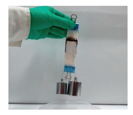
Fig. 6 Photograph of two pieces of porcine skin bonded together with an Alg–DA hydrogel showing that they are able to support 300 g weight. Overlapped area:  $25 \text{ mm} \times 25 \text{ mm} \times 1 \text{ mm}$ .
