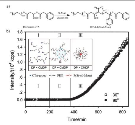
Fig. 3 (a) RAFT dispersion copolymerization of styrene and maleic anhydride in chloroform with a PEO macro-CTA. (b) Time dependence of the scattering intensity of the polymerization system at scattering angles of 30° and 90°. The inset shows three respective stages during the polymerization-induced self-assembly process.12
