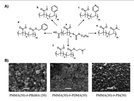
Fig. 13 (A) The block copolymers synthesized by RAFT dispersion polymerization in scCO<sub>2</sub> from PMMA-RAFT precursors (a): PMMA-b-PSt (b), PMMA-b-P4VP (c), PMMA-b-PBZMA (d), PMMA-b-PDMA (e), PMMA-b-PDMAEMA (f). (B) SEM of the block copolymer particles. Scale bar in each image is 5 μm.<sup>34</sup>
