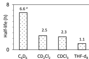
**Figure 4.** Impact of solvent on the lifetime of **GIm** (18 mM) at 35 °C. Assessed by <sup>1</sup>H NMR analysis; integration against TMB as internal standard. <sup>a</sup> Cf. reported half-life at 55 °C in C<sub>6</sub>D<sub>6</sub>: 40 min.<sup>33</sup>
