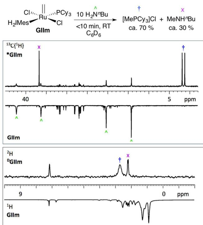
**Figure 5.** Spectra showing the superior rapidity and clarity with which  $^{13}\text{C}$ -labelling enables tracking of the methylidene moiety during decomposition. Top:  $^{13}\text{C}\{^1\text{H}\}$  NMR spectra; 20 min acquisition for **\*GIIm** and (inverted) 5.5 h acquisition for non-enriched **GIIm**. Bottom:  $^2\text{H}$  spectrum for **DGIIm** and (inverted)  $^1\text{H}$  NMR spectrum for **GIIm** (2 h and 5 min acquisition, respectively).
