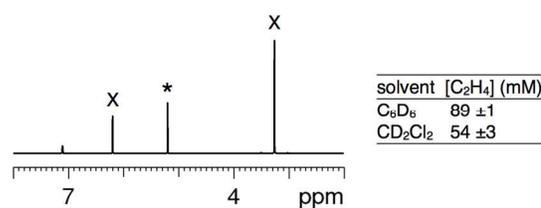
**Figure 3.** Measuring the solubility of ethylene in organic solvents by <sup>1</sup>H NMR analysis (300.1 MHz). Left: representative spectrum. Signal labelled (\*) is due to C<sub>2</sub>H<sub>4</sub>, (X) denotes TMB; C<sub>6</sub>HD<sub>5</sub> signal not labelled. Right: tabulated data. Conditions: 296 ± 1.5 K, 101.0 ± 0.8 kPa, 5 x freeze-pump-thaw cycles prior to equilibrating under ethylene; experiments in triplicate.
