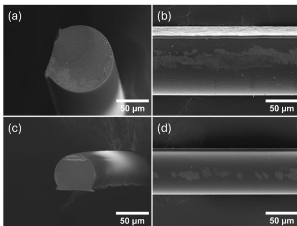
Fig. 1 SEM images of air-dried as-spun Kraft lignin–PVA fibres spun continuously from [DMBA][HSO<sub>4</sub>] and water mixtures using a 25 G (260 μm) spinneret (a and b) and a 30 G (159 μm) spinneret (c and d).
