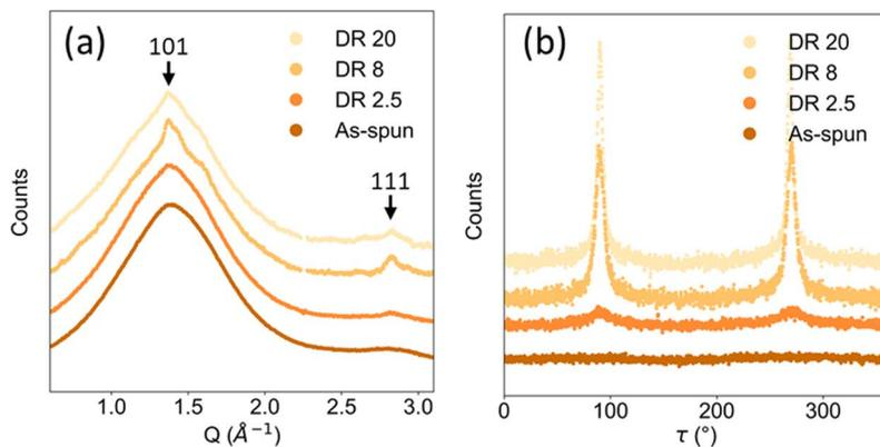
Fig. 5 (a) Scattering diagrams and (b) angular modulation of the intensity at  $Q = (1.39 \pm 0.04) \text{ \AA}^{-1}$  for the as-spun and hot-drawn 25 G fibres. Position of diffraction peaks of crystalline PVA are indicated with arrows and their Miller indices are provided. Curves are translated vertically for the sake of clarity.
