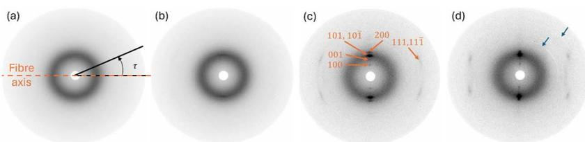
Fig. 4 WAXS patterns of 25 G as-spun lignin–PVA fibres (a), and lignin–PVA fibres hot-drawn at  $180 \text{ }^\circ\text{C}$  to DR 2.5 (b), DR 8 (c), and DR 20 (d). The blue arrows highlight artefact rings resulting from the background subtraction. Miller indices of diffraction peaks of crystalline PVA are provided in (c).
