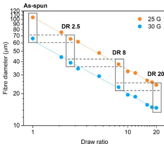
Fig. 3 Relationship between fibre diameter and ratio for lignin–PVA fibres extruded through 25 G (260  $\mu\text{m}$ ) and 30 G (159  $\mu\text{m}$ ) spinnerets. Vertically oriented boxes indicate fibres with the same draw ratio (but different diameter) and horizontally oriented boxes (dashed) indicate hot-drawn fibres with the same diameter (but different draw ratios). The orange and blue lines (dotted) fitted to the 25 G and 30 G data have slopes of  $-0.49$  and  $-0.50$ , respectively.
