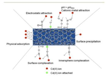
Fig. 4 Schematic showing the interaction of Cd(II) ions with Al<sub>2</sub>O<sub>3</sub>/ MWCNTs.30
