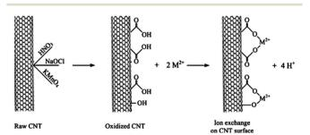
Fig. 3 Adsorption mechanism of heavy metals on CNTs with COOH and OH groups. 43
