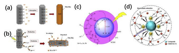
Fig. 6 Mechanisms of heavy metal ion removal using ZnO or TiO<sub>2</sub> particles *via* (a) adsorption on ZnO (ref. 83), (b) reduction/oxidation process on ZnO (ref. 83) and (c) photocatalysis on TiO<sub>2</sub> (ref. 82). d) Potential reactions involved in the adsorption of metal ions by magnetic iron oxide nanoparticles.<sup>84</sup>
