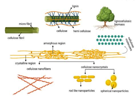
Fig. 8 Extraction and preparation sequences for cellulose nanocrystals (CNC) and cellulose nanofibers (CNF).<sup>22</sup>
