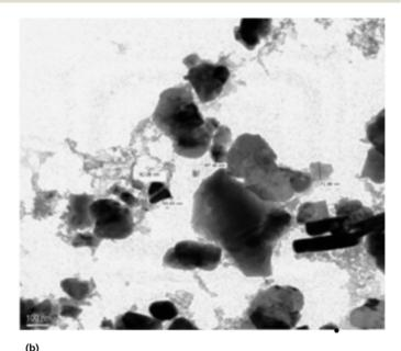
Fig. 12 a) SEM micrograph and b) TEM micrograph of nanocomposite ZrO<sub>2</sub>/B<sub>2</sub>O<sub>3</sub>. <sup>133</sup>
