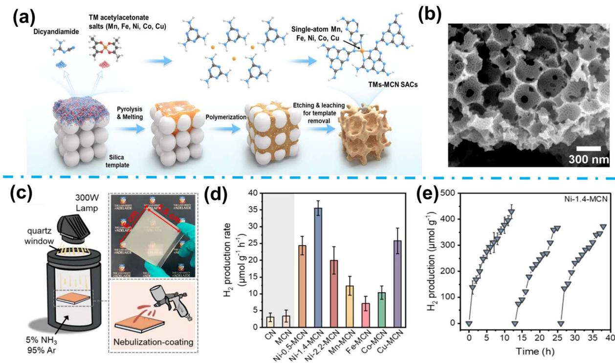
Fig. 3 (a) Schematic illustration of the fabrication process of TMs-MCN SACs. (b) SEM. (c) Schematic illustration of the reaction system and nebulization-coating method. (d)  $\text{H}_2$  production rates of CN, MCN, and Ni-MCNs with different Ni loadings and TMs-MCNs and (e) cycling tests.<sup>58</sup> Copyright 2023, American Chemical Society.
