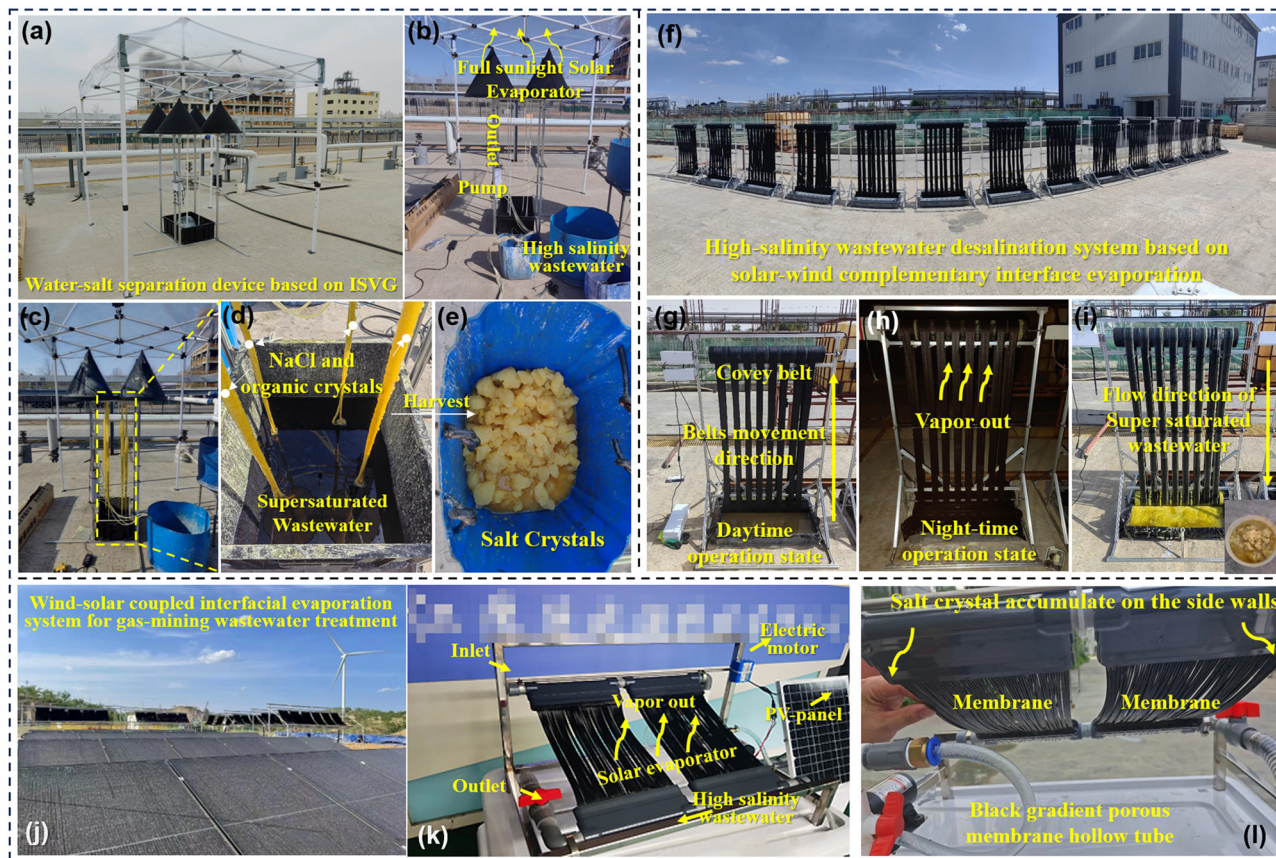
Fig. 36 Commercially available salt collection-oriented devices based on ISVG technology. (a) Comprehensive view of the conical high-salinity desalination device; (b) Diagram showing the salt extraction rope and conical evaporator; (c) and (d) high-salinity wastewater being pumped into the conical evaporator; (e) collection of crystalline salt after evaporation; (f) comprehensive view of the solar-wind complementary system equipment; (g) day-time and (h) night-time operation state of a single unit; (i) high-salinity wastewater concentration operation state of a single unit (insert: salt crystals collected by the equipment after concentrating high-salinity wastewater). (j) Comprehensive view of the zero-liquid discharge equipment for high-salinity mining wastewater treatment. (k) and (l) Diagram of the graphene black crystal membrane for solar evaporation. Our group work, Product Copyright @ Xi'an Qinshengfeng Tech. Co. Ltd, Photo copyright @ author Yawei Yang, All rights reserved; (j)–(l) Copyright from Jiangsu Juzhilian Technology Co., Ltd, all rights reserved.
