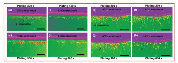
Fig. 13 Operando SEM images of the Li/Cu anode used by Rong et al. at increasing plating times for a solution containing (a)–(d) 0.2 M Li<sub>2</sub>S<sub>8</sub> and (e)–(h) 0.2 M Li<sub>2</sub>S<sub>8</sub> with 1 wt% LiNO<sub>3</sub>. Scale bar: 10  $\mu$ m ((a)–(h) adapted with permission from ref. 135, Copyright (2017) Wiley-VCH.)
