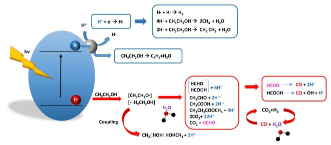
Fig. 2 Schematic representation of the radical species and intermediates detected in the photocatalytic production using ethanol as a sacrificial molecule. Colour codes are explained in the text.
