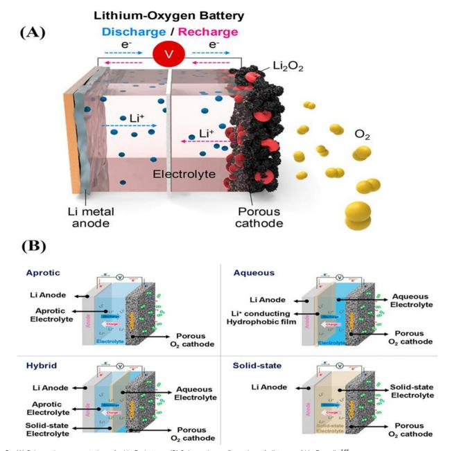
Fig. 9 (A) Schematic representation of a  $Li-O_2$  battery. (B) Schematic configuration of all types of  $Li-O_2$  cells. <sup>145</sup>
