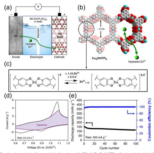
Fig. 10 Cu<sub>3</sub>(HHTP)<sub>2</sub> acting electrochemically as a cathode for rechargeable ZIBs. (a) Zn-Cu<sub>3</sub>(HHTP)<sub>2</sub> cell schematic depiction. (b) The Cu<sub>3</sub> (HHTP)<sub>2</sub> chemical structure. (c) The anticipated redox mechanism in the  $Cu_3$  coordination unit (HHTP)<sub>2</sub>. (d) CV profile at 0.5 mV s @1, together with the capacitive contribution (shaded region). (e) Cycling efficiency at 500 mA g @1.157
