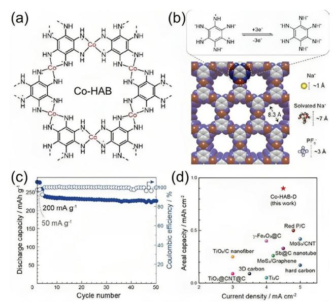
Fig. 8 Electrochemical performance of the Co-HAB electrode for SIBs. (a) Chemical structure of Co-HAB. (b) A space-filling diagram of Co-HAB and the size comparison of the pore with  $Na^+$ , solvated  $Na^+$  and  $PF_6$ @ions. Top: proposed three-electron reversible reaction of the HAB ligand in Co-HAB. (c) Cycling stability test of the Co-HAB electrode. (d) Comparison of areal capacity of Co-HAB with representative reported anode materials for SIBs. 137
