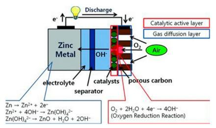
Fig. 11 Working principle and each electrode reaction of zinc-air batteries. Note the red circle where a three phase reaction (oxygen (gas), catalysts (solid) and electrolyte (liquid)) occurs in the air cathode. 174
