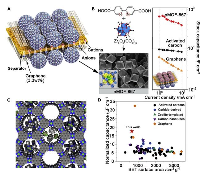
Fig. 3 MOF-based supercapacitors. (A) Schematic construction of MOF supercapacitors. <sup>53</sup> (B) Structure and nanocrystal morphology of nMOF-867 and comparison of stack capacitances among various EDLC materials. 51 (C) A space-filling diagram of idealized Ni<sub>3</sub>(HITP)<sub>2</sub> (Ni, green; F, lime; N, blue; C, gray; B, brown; H, white).<sup>51</sup> (D) Comparison of BET-surface-area-normalized areal capacitances among various EDLC materials.<sup>54</sup>
