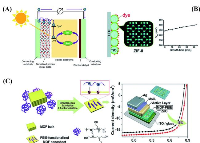
Fig. 4 (A) Schematic representation of typical dye-sensitized solar cells. (B) The use of MOFs for the photoanodes in DSSCs as the blocking layer. (C) Schematic illustration of the preparation of 2D MOF nanosheets and their modified electron-extraction layer for photovoltaic devices.<sup>72</sup>
