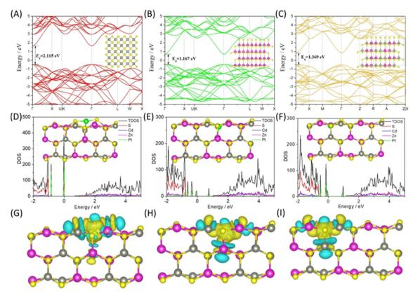
Fig. 12 The electronic structures of (A) ZnS, (B) CdS, and (C) Zn<sub>x</sub>Cd<sub>1-x</sub>S are shown (the gray, pink, and yellow spheres represent Zn, Cd, and S atoms, respectively). The work functions of (D) ZnxCd1@xS-Pt1, (E) ZnxCd1@xS-Pt1 (Zn), (F) ZnxCd1@xS-Pt1 (Cd). (G), (H), and (I) indicate the DOSs and charge density differences. 139
