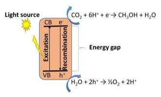
Fig. 7 Schematic representation of a single photocatalyst.
