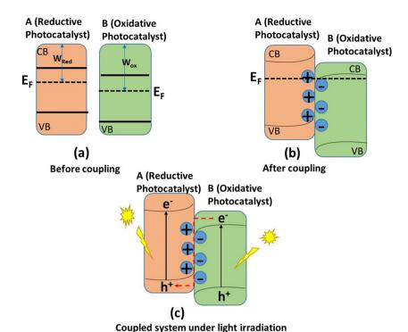
Fig. 9 The mechanism of direct Z-scheme photocatalyst production using oxidative and reductive semiconductors, showing the band structures (a) before and (b) after coupling. (c) The band structure of a linked system under light irradiation. The Fermi energy level is denoted by the symbol  $E_E$ .
