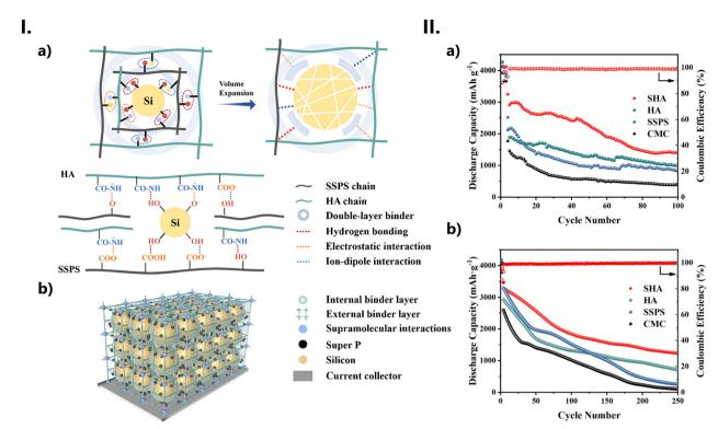
Fig. 22 (I) (a) Schematic diagram of the double-layer binder network resisting against volume expansion and illustration of supramolecular interactions between HA and Si NPs. (b) 3D network of Si anodes with HA as binder. (II) Cycling performance of various binders at (a) 4 A g<sup>-1</sup> and (b) 2 A g<sup>-1</sup>. Reproduced from ref. 222 with permission from Elsevier; copyright © 2018 Elsevier B.V.
