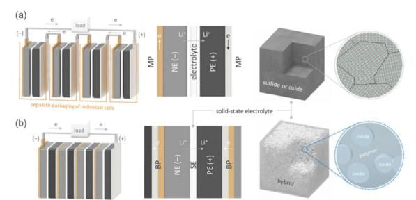
Fig. 10 Schematic diagrams of (a) the monopolar design of current LIBs with liquid electrolytes and (b) bipolar design of SSLBs equipped with SEs. The Li<sup>+</sup> and electron pathways during discharge are also indicated. (Reproduced with permission from ref. 63)
