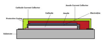
**Fig. 9** Cross-section of a thin-film solid-state battery showing different components. The substrate acts as a support on which the thin film is usually deposited. (Reproduced with permission form ref. 37).
