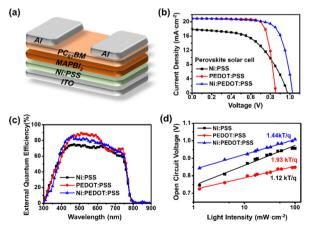
Fig. 1 (a) Device structure of p-i-n perovskite solar cells, (b) J-V characteristics, (c) external quantum efficiency spectra, and (d) light dependence of perovskite solar cells with Ni:PSS, PEDOT:PSS and PEDOT:PSS-doped Ni:PSS HTLs.
