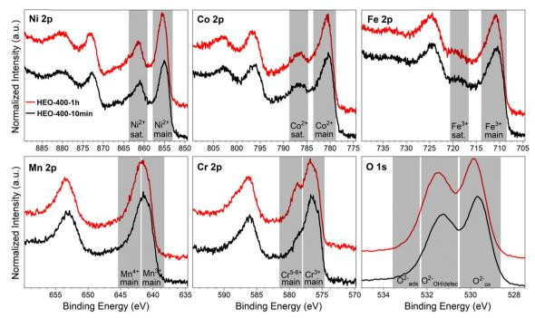
Fig. 2 2p core level photoemission spectra of Ni, Co, Fe, Mn, Cr, and O for the HEO-400-10min (black) and HEO-400-1h (red) thin films acquired at a constant kinetic energy of 610 eV with grey areas indicating commonly assigned speciation/oxidation state ranges.
