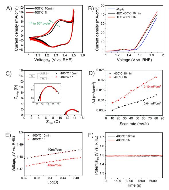
Fig. 3 Electrochemical performance of HEO-400-10min (black) and HEO-400-1h (red): (A) cyclic voltammetry curves, (B) linear sweep voltammetry, (C) Nyquist plots measured at 1.6 V vs. RHE, (D) differential current densities and the corresponding the double-layer capacities, CDL, determined by linear fitting, (E) Tafel plots, and (F) chronopotentiometry analysis performed at 10 mA cm<sup>-2</sup> for 2 hours. All experiments were conducted in 1 M KOH  $(pH \approx 13.6)$
