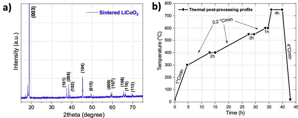
Fig. 4 (a) XRD diffractogram obtained from the residues left from thermal post-processing. The reflections of  $\text{LiCoO}_2$  are indicated in parentheses. (b) Thermal post-processing profile including debinding and sintering steps.
