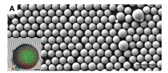
Fig. 13 Scanning electron microscope (SEM) image of self-assembled core-shell SiO2@TiO2@PS nanoparticles (NPs) after deposition on the silicon wafer (down left frame). Scale bar 1.5 μm (figure from Cossi et al.<sup>65</sup> work).
