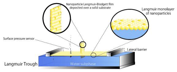
Fig. 8 Typical LB experiment of a deposition of a nanoparticle Langmuir film.
