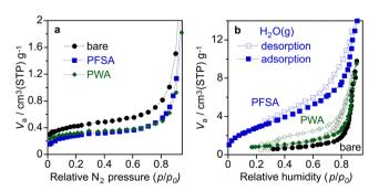
Fig. 6 (a) Nitrogen adsorption isotherms at -196 °C and (b) water vapour adsorption-desorption isotherms at 25 °C for bare WO<sub>3</sub>, PWA/WO<sub>3</sub>, and PFSA/WO<sub>3</sub> layers on Ti felt. The loading of PWA and PFSA were 5 and 12 wt% relative to WO3.
