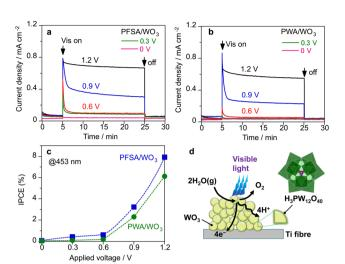
Fig. 5 Effect of applied voltage (V vs. Pt-CB cathode) on the photocurrent response of (a) PFSA/WO<sub>3</sub> and (b) PWA/WO<sub>3</sub> in the vapour-fed PEM-PEC system under visible light (453 nm, 22 mW cm<sup>-2</sup>). (c) Steady-state IPCE at 453 nm after 20 min of photoirradiation. (d) Schematic illustration of PEC triple-phase boundary over the PWA/WO<sub>3</sub> photoanode. The loading of PWA and PFSA were 5 and 12 wt% relative to WO3.
