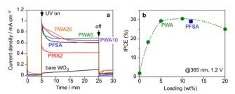
Fig. 4 Photocurrent response of the WO<sub>3</sub> photoanodes in a continuous flow of humidified argon (RH < 90%) under UV irradiation (365 nm, 7.0 mW cm $^{-2}$ , area 2 cm $^{2}$ ). (a) Photocurrent response of WO $_{3}$  photoanodes coated with PFSA and PWA with different loading amount (wt%) at 1.2 V vs. Pt-CB cathode. (b) Incident photon-to-current conversion efficiency (IPCE) at 1.2 V.
