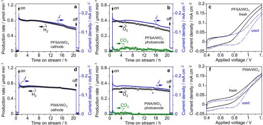
Fig. 7 Long-term stability test of (a) – (c) PFSA/WO<sub>3</sub> and (d) – (f) PWA/WO<sub>3</sub> photoanodes in the vapour-fed PEM-PEC system under visible light (453 nm, 12 mW cm<sup>-2</sup>, area 16 cm<sup>2</sup>) at 1.2 V (vs. Pt-CB): (a) and (d) Production rate of H<sub>2</sub> in the cathode side, (b) and (e) production rate of O<sub>2</sub> and CO<sub>2</sub> in the photoanode side, and (c) and (f) cyclic voltammograms before and after the stability test.
