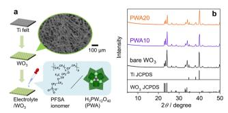
Fig. 1 (a) Preparation of porous WO<sub>3</sub> photoanode and surface electrolyte coating. (b) XRD patterns of PWA/WO<sub>3</sub> photoanodes and the standard lines of  $WO_3$  (JCPDS No. 01-072-0677) and Ti (JCPDS No. 00-044-1294).
