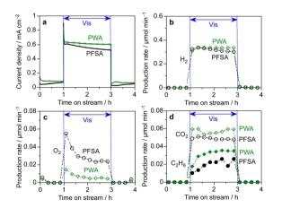
Fig. 8 PEM-PEC methane conversion reactions using the PWA/WO<sub>3</sub> and PFSA/WO<sub>3</sub> photoanodes at 1.2 V (vs. Pt-CB) under visible light irradiation (453 nm, 22 mW cm $^{-2}$ , and area 2 cm $^{2}$ ): (a) photocurrent response, (b) H<sub>2</sub> production rate at the cathode, (c) O<sub>2</sub> production rate at the photoanode and (d) production rate of CO<sub>2</sub> and C<sub>2</sub>H<sub>6</sub> at the photoanode.
