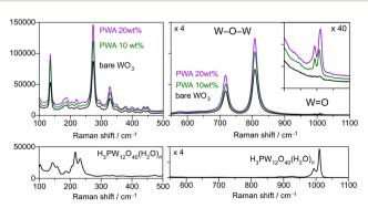
Fig. 2 Raman spectra of the WO<sub>3</sub> photoanodes with and without the PWA (10 and 20 wt%) coating and H<sub>3</sub>PW<sub>12</sub>O<sub>40</sub>·nH<sub>2</sub>O crystalline powder.
