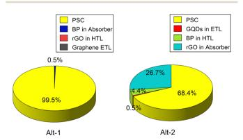
Fig. 3 The breakdown of environmental impacts by each component of Alt-1 and Alt-2 ld-PSC on overall average impacts. The environmental impacts of each component for 1 m<sup>2</sup> of the ld-PSC module were calculated for all impact categories. The average contribution of each component is calculated according to Celik et al. 78 The raw data for each component for 1 m<sup>2</sup> is also provided in Tables S.2-S.5 (ESI†).
