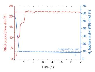
Fig. 2 Productivity and H2 fraction in SNG at the reactor outlet at the start-up of the biogas methanation plant (experimental conditions: 8 bar,  $H_2$ :  $CO_2$  = 4.15, cooling setpoint = 230 °C). The  $CO_2$  conversion is 100% in the entire time interval considered and no other products than methane were observed
