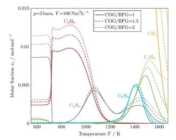
Fig. 6 Kinetic simulation of coke precursors and methane at constant reactor wall temperatures for 3 different COG/BFG ratios.
