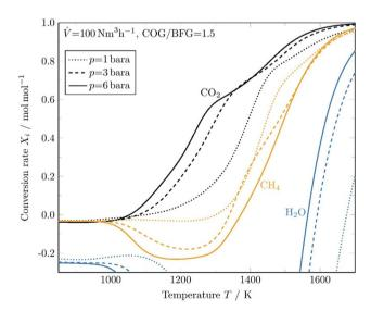
Fig. 4 Simulated conversion rates as function of temperature at three different pressure levels predicted by DETCHEMCHANNEL
