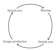
Scheme 3 Sequence of the cyclic operation of the pilot plant.
