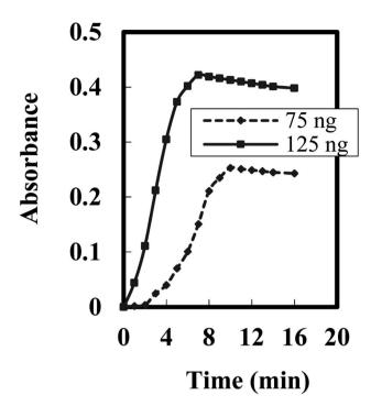
Fig. 4 Steady state response time of the optode towards different  $[Cr(v_1)] - 75 \text{ ng mL}^{-1} \text{ and } -125 \text{ ng mL}^{-1}$ .
