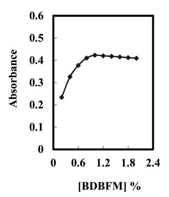
Fig. 3 Effect of the BDBFM percentage on the optode membrane immersed in 125 ng mL<sup>-1</sup> of Cr(vi) under optimum conditions.
