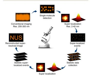
Fig. 1 Schematic illustrating the principles of single-molecule fluorescence imaging.
