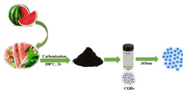
Fig. 5 A schematic illustration of the synthesis of water-soluble fluorescent CQDs from watermelon peels. 46
