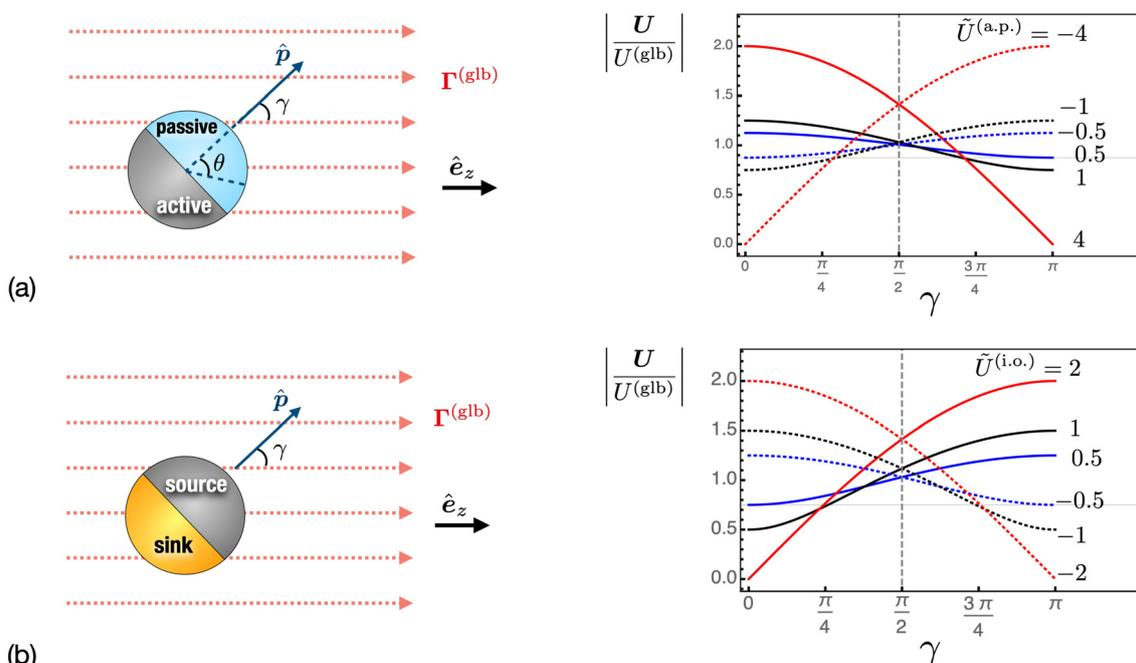
Fig. 2 Two self-phoretic Janus models of (a) active-passive (a.p.) and (b) sink-source (i.o.) composition are undergoing globally-driven phoresis by the far-field flux  $\Gamma^{(\text{glb})}$ . The angle  $\gamma$  defines the orientation of the Janus director  $\hat{p}$  with respect to  $\Gamma^{(\text{glb})}$ . Solid lines represent positive values of  $\tilde{U}^{(\alpha)}$ , while dashed lines represent negative values.
