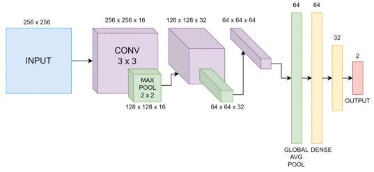
Fig. 1 Example sequential CNN architecture, including layer output dimensions. "CONV" represents a 3 × 3 convolutional layer and "MAX POOL" and "GLOBAL AVG POOL" maximum and global average pooling
