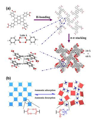
Fig. 8 (a) Crystal structures of FDU-HOF-3; (b) schematic illustration of the self-healing effect of FDU-HOF-3 before and after  $NH_3$  capture.<sup>64</sup>
