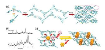
Fig. 15 (a) Assembling of PTTCN molecules (left) to a 2D H-bonded framework with pores (middle), and intermolecular stacking in a 2  $\times$  2 cell (right); (b) PXRD patterns; (c) schematic representation of the separation for benzene/cyclohexane.<sup>93</sup>
