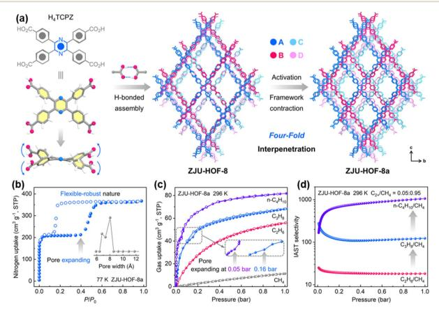
Fig. 13 (a) Single-crystal structure of ZJU-HOF-8 and the structural transformation with framework contraction upon activation; (b)  $N_2$  adsorption of ZJU-HOF-8a at 77 K; (c) different gas adsorption at 296 K; (d) IAST selectivities of ZJU-HOF-8a at 296 K.55
