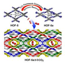
Fig. 5 Illustration of the structural deformation of HOF-5 and the arrangement of CO<sub>2</sub> molecules in the pores.<sup>45</sup>
