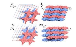
The AA stacking pattern of HOF-29 viewed perpendicularly (a) and side views (b); the AB stacking pattern of HOF-29⊃pX viewed perpendicularly (c) and side views (d).57
