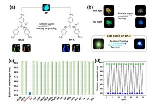
Fig. 16 (a) Tautomerism of BA-N and BA-C; (b) images showing reversible switching between BA-N and BA-C ( $\lambda_{\rm ex}=365$  nm), as well as LED light-emitting images before and after acetone fumigation; (c) histogram of the prompt emission peaks of BA-N following fumigation; (d) repeatability of luminescence color switching when stimulated with acetone vapor and heated.<sup>68</sup>
