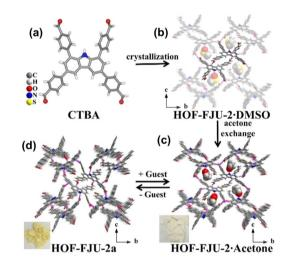
Fig. 11 (a) The tetrabenzaldehyde molecule CTBA; (b) structure of HOF-FJU-2·DMSO; (c) HOF-FJU-2·Acetone; (d) reversible SCSC transformation after guest removal to nonporous HOF-FJU-2a.66
