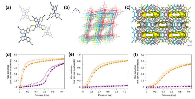
Fig. 6 (a) The intermolecular H-bonding interactions between bicarbazole units; (b) the threefold-interpenetrated dia net; (c) pore channels along the [100] direction; (d-f) gas adsorption isotherms for  $C_2H_4$  (orange) and  $C_2H_6$  (purple) at 298 K, 318 K and 333 K, respectively.
