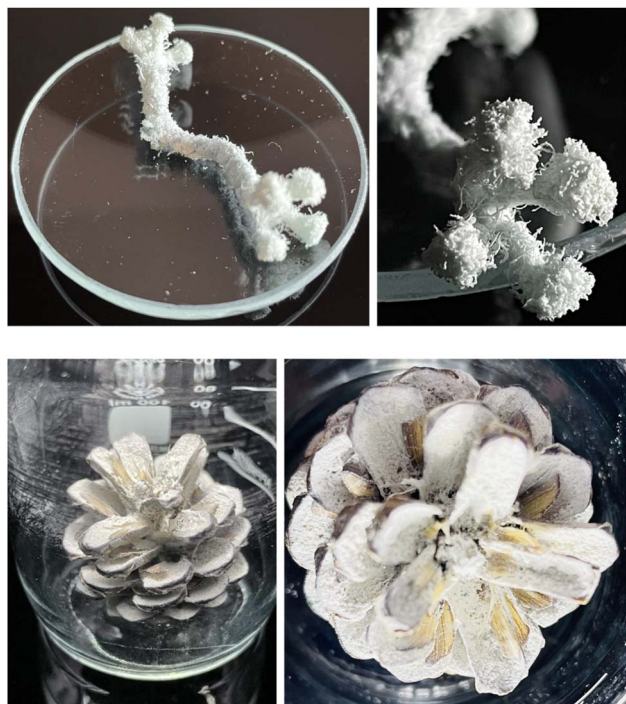
Fig. 7 A cotton thread (top) and a pine tree cone (bottom) grafted with poly(MMA) via the two step TAI-modification/ATRP-grafting strategy.
