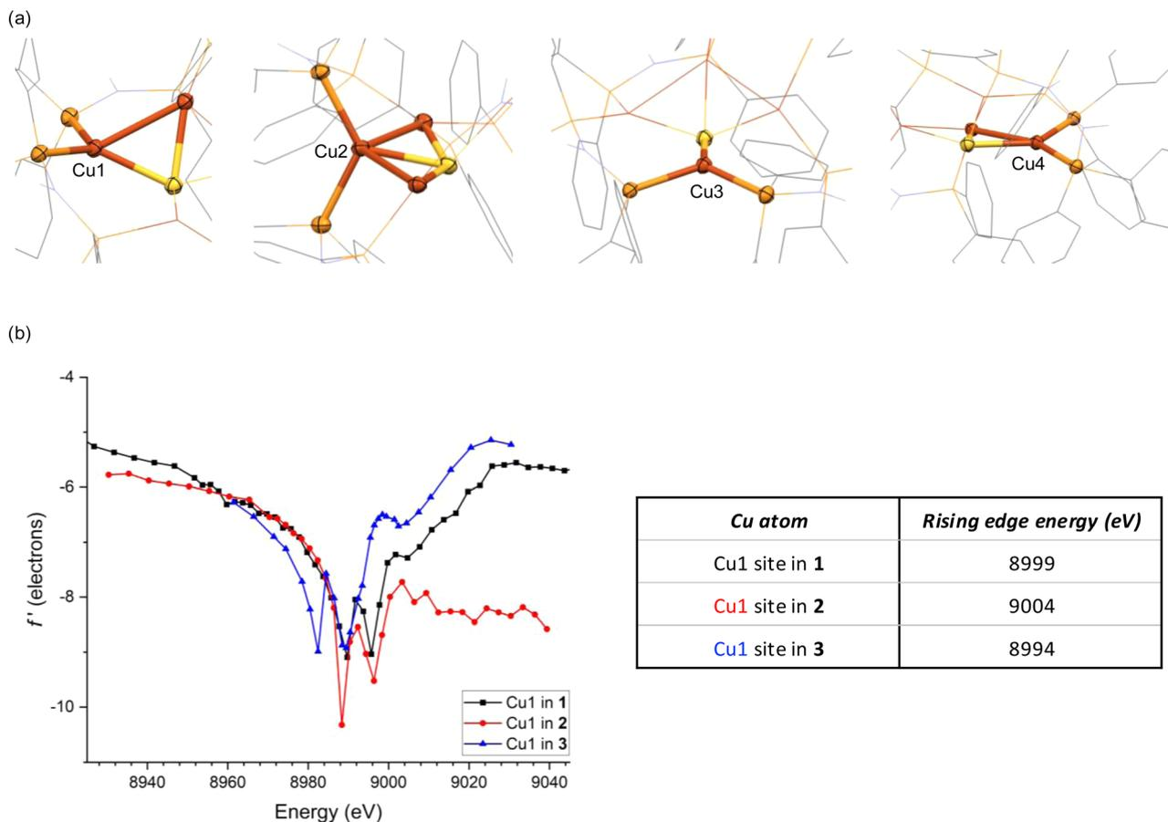
Fig. 3 (a) Nearest neighbor atoms surrounding each Cu site in **1**; (b) DAFS data for the Cu1 sites in **1**, **2**, and  $[\text{Cu}_2(\text{dppa})_2][\text{PF}_6]_2$  (**3**). Rising edge energies were estimated using a linear regression protocol described in ESI.†
