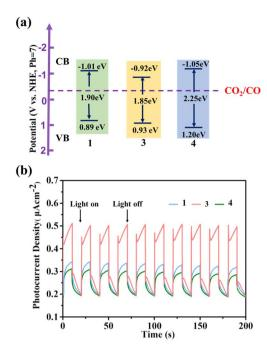
Fig. 6 (a) Energy-level diagram of 1, 3 and 4; (b) 0.4 V-bias photo-current responses of electrodes derived for 1, 3 and 4 in  $0.2 \text{ M Na}_2\text{SO}_4$  aqueous solution under repetitive chopped visible light irradiation.
