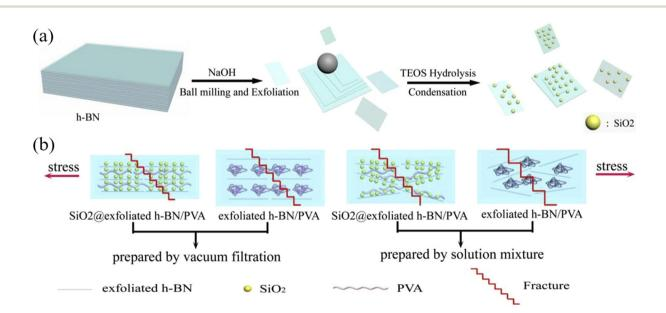
Fig. 35 (a) Preparation of boron nitride nanosheets and SiO<sub>2</sub>@BN bybrids. (b) Fracture behaviour of PVA composites with h-BN and SiO<sub>2</sub>@h-BN prepared by solution casting and vacuum filtration. Reproduced with permission from ref. 384. Copyright 2018 Elsevier.
