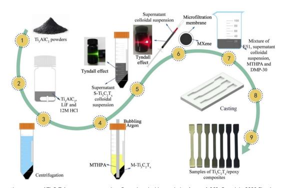
$\textbf{Fig. 28} \quad \text{Preparation process of $Ti_3C_2T_x$/epoxy nanocomposites. Reproduced with permission from ref. 262. Copyright 2020 Elsevier.}$
