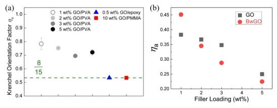
Fig. 18 (a) Krenchel orientation factors of GO/PVA, GO/epoxy and GO/PMMA nanocomposites. Reproduced with permission from ref. 167. Copyright 2016 Elsevier. (b) Variations of agglomeration factor with GO and BwGO (the functional groups of GO were partially removed by base wash) filler loadings. Reproduced with permission from ref. 170. Copyright 2018 Elsevier.
