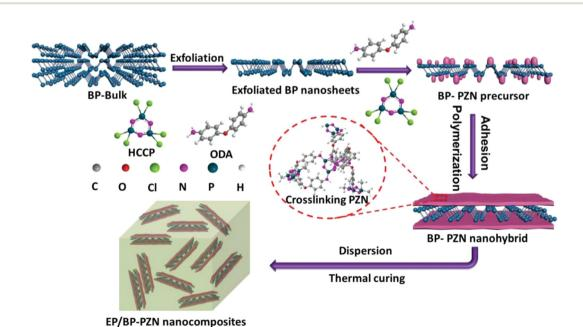
Fig. 30 Preparation of PZN-functionalized BP nanosheets and BP/epoxy nanocomposites. Reproduced with permission from ref. 289. Copyright 2019 WILEY-VCH Verlag GmbH & Co. KGaA.
