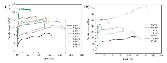
Fig. 20 Variations of stress-strain curves with filler loading for (a) GO/PVA and (b) rGO/PVA nanocomposites, respectively. Reproduced with permission from ref. 175. Copyright 2011 Wiley-VCH Verlag GmbH & Co. KGaA.
