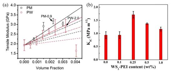
Fig. 27 (a) Tensile modulus for the PVA composites based on  $MoS_2$  (PM) and  $WS_2$  (PW). Reproduced with permission from ref. 245. Copyright 2014 Royal Society of Chemistry. (b) Variation of facture toughness of  $WS_2$ /epoxy composites with volume fraction. Reproduced with permission from ref. 246. Copyright 2017 American Chemical Society.
