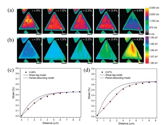
Fig. 8 PL A exciton (a) intensity and (b) peak mapping of  $MoS_2$  with applied strain increasing from 0 to 4.8%. (Scale bar, 4  $\mu$ m). Reproduced with permission from ref. 114. Copyright 2014 Nature Publishing Group. Strain distribution in monolayer  $MoS_2$  at (c) 0.46% and (d) 0.67% strain. Both shear-lag model and partial-debonding model were used to fit the experimental results. Reproduced with permission from ref. 115. Copyright 2023 Elsevier.
