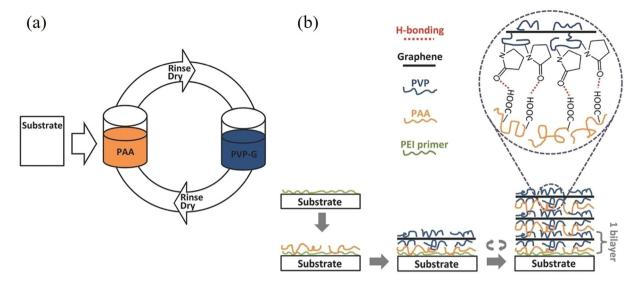
Fig. 16 Layer-by-layer assembly for the preparation of graphene/polymer composites. Reproduced with permission from ref. 163. Copyright 2016 Wiley-VCH Verlag GmbH & Co. KGaA.
