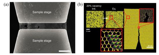
Fig. 4 (a) Suspended monolayer graphene over a tension stage for fracture toughness measurement. Scale bar,  $5 \mu m$ . Reproduced with permission from ref. 81. Copyright 2014 Nature Publishing Group. (b) Crack propagation in monolayer  $MoS_2$  with line defects. Reproduced with permission from ref. 82. Copyright 2016 American Chemical Society.
