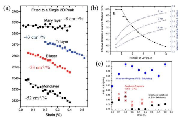
Fig. 10 (a) Raman 2D shifts of monolayer, bilayer, trilayer and multilayer graphene in a polymer/graphene/polymer model composite. (b) Variations of effective elastic modulus of graphene with layer number. Reproduced with permission from ref. 128. Copyright 2012 American Chemical Society. (c) Interfacial shear stress of graphene–polymer and graphene–graphene. Reproduced with permission from ref. 129. Copyright 2020 Nature Publishing Group.
