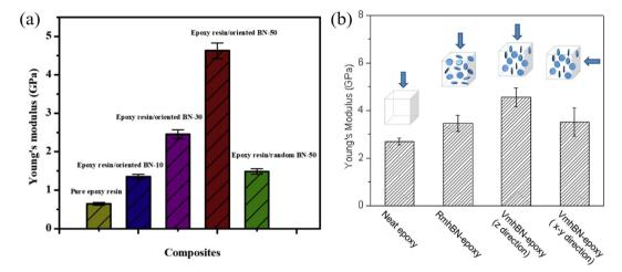
Fig. 25 (a) Variation of the Young's modulus of the h-BN/epoxy nanocomposites with h-BN content. Reproduced with permission from ref. 219. Copyright 2018 Elsevier. (b) Variation of the Young's modulus of h-BN/epoxy nanocomposites with the orientation of h-BN. Reproduced with permission from ref. 220. Copyright 2013 American Chemical Society.
