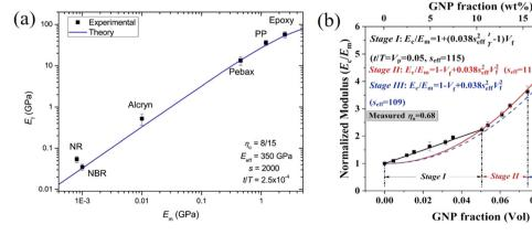
Fig. 19 (a) Variation of the modulus of graphene nanoplatelets (GNPs) with the modulus of the matrices (dots: experiment data; blue line: theory predictions from eqn (16) and (19)). Reproduced with permission from ref. 171. Copyright 2018 Elsevier. (b) Three stages for the reinforcement of GNPs on elastomers. Reproduced with permission from ref. 153. Copyright 2019 Elsevier.
