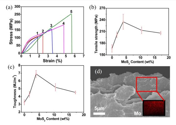
Fig. 32 (a) Stress-strain curves of GO/MoS<sub>2</sub>/TPU nanocomposites. 1 to 5 represent GO film, GO/TPU, rGO/TPU, GO/MoS<sub>2</sub>/TPU, and rGO/MoS<sub>2</sub>/ TPU composites, respectively. Dependence of the (b) tensile strength and (c) toughness of the composites with the loading of MoS<sub>2</sub>. (d) Fracture surface of the rGO/MoS<sub>2</sub>/TPU composites. Reproduced with permission from ref. 317. Copyright 2015 American Chemical Society.
