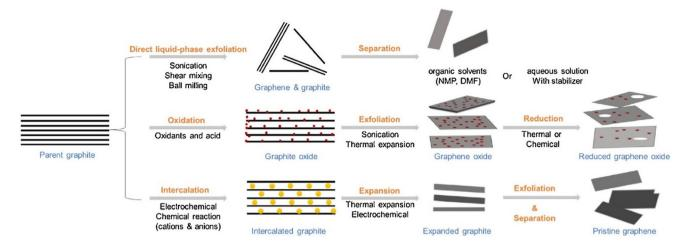
Fig. 2 Liquid exfoliation methods for the preparation of graphene and related 2D nanosheets, including mechanical force-assisted, oxidationassisted and intercalation-assisted exfoliation. Reproduced with permission from ref. 11. Copyright 2018 Elsevier.
