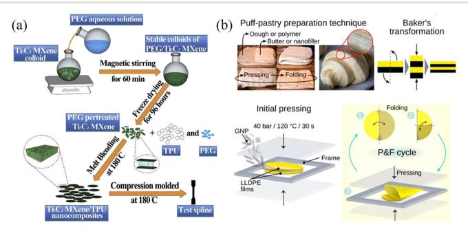
Fig. 14 (a) Melt mixing method for the preparation of MXene/TPU composites. Reproduced with permission from ref. 149. Copyright 2019 Elsevier. (b) Puff-pastry preparation inspired pressing-and-folding method and illustration of this method for the fabrication of a GNP/LLDPE composite film. Reproduced with permission from ref. 155. Copyright 2018 America Chemical Society.
