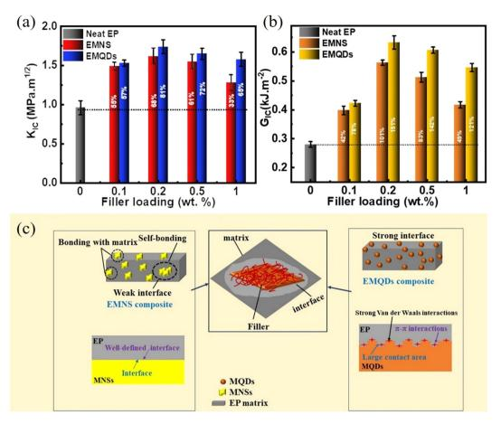
Fig. 26 (a)  $K_{IC}$  and (b)  $G_{IC}$  of neat epoxy, epoxy/MNSs (EMNS) and epoxy/MQDs (EMQDs) nanocomposites. (c) Interfacial interactions of EMNS and EMQDs. Reproduced with permission from ref. 241. Copyright 2021 Elsevier.
