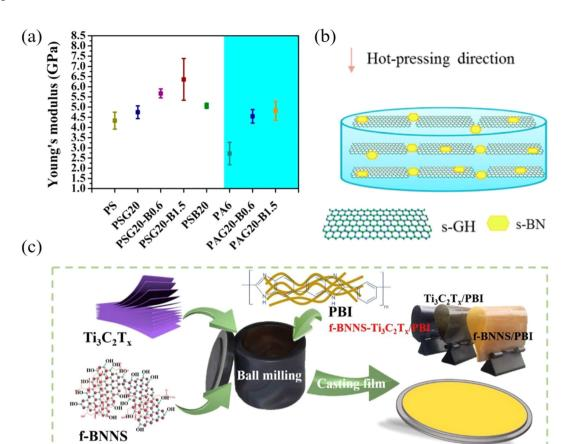
Fig. 31 (a) Variation of the Young's modulus of PS and PA composites with the addition of graphene and BN. (b) Scheme for the stacking of graphene (s-GH) and BN (s-BN). Reproduced with permission from ref. 311. Copyright 2015 American Chemical Society. (c) Preparation process of PBI-based composite films. Reproduced with permission from ref. 319. Copyright 2019 Elsevier.
