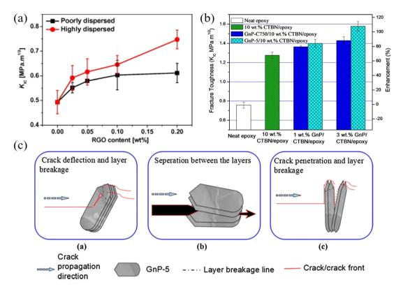
Fig. 22 (a) Variations of K<sub>IC</sub> of rGO/epoxy nanocomposites with rGO loading. Reproduced with permission from ref. 178. Copyright 2013 Elsevier. (b) Effects of CTBN and GNP on the fracture toughness of epoxy composites. (c) Crack propagation in GnP-5 flakes. Reproduced with permission from ref. 179. Copyright 2016 Elsevier.
