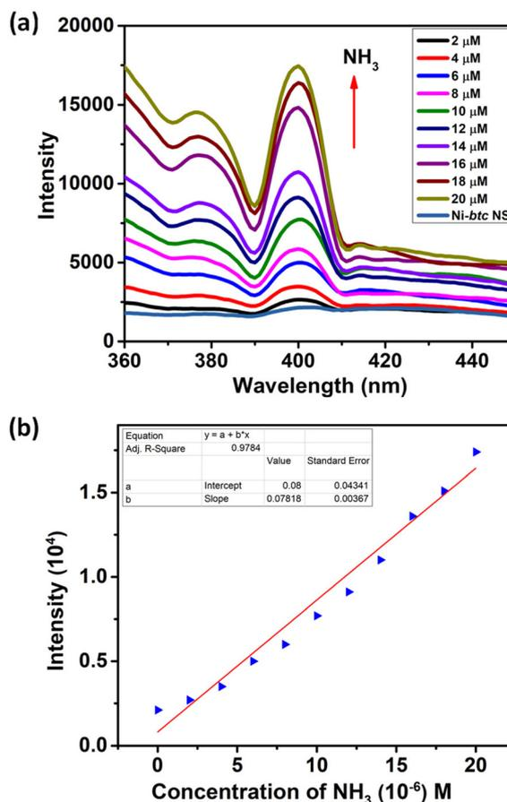
**Fig. 2** (a) Emission spectrum of Ni-*btc* NS dispersed in water showing increase in intensity upon gradual addition of ammonia solution. (b) Determination of LOD via linear fitting of the fluorescence intensity of Ni-*btc* NS upon adding different concentrations of ammonia solution at  $\lambda_{\text{emi}} = 400 \text{ nm}$  (upon  $\lambda_{\text{exc}} = 310 \text{ nm}$ ).
