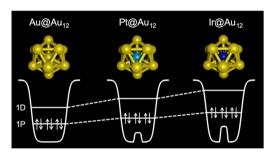
**Fig. 1** Schematic illustration of the two-step jellium potential and superatomic orbitals of  $M@(Au^+)_{12}$  ( $M = Au^+, Pt^0, Ir^-$ ). Reproduced from ref. 95 with permission from the American Chemical Society, Copyright 2020
