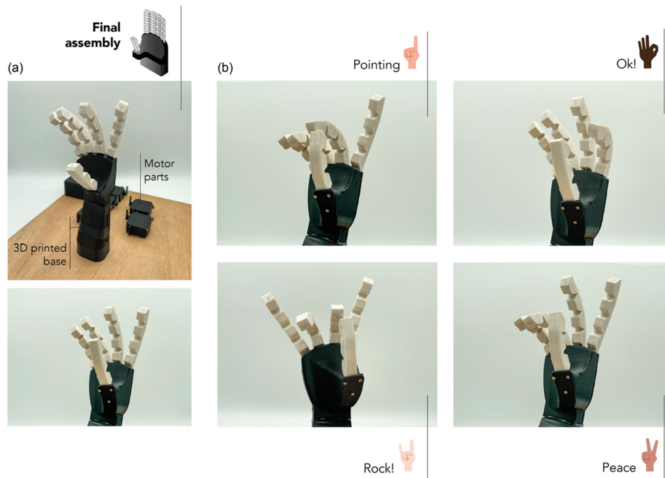
Fig. 10 (a) Final assembly of gripper and (b) actuation of four programmed positions (pointing, ok, rock, and peace signs).
