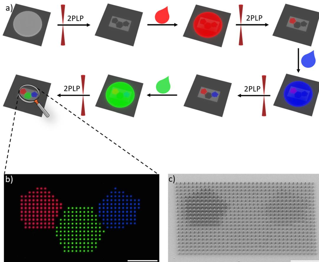
**Fig. 6** (a) A schematic workflow to fabricate RGB emissive pixel like pillars. (b) Multi-material print of pixel like pillars. The *via* confocal microscopy recorded RGB channels were combined to create the depicted image. (c) Tilted SEM image of the same structure as in b (Scalebars = 20  $\mu\text{m}$ ).
