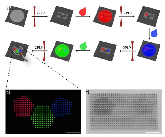
Fig. 6 (a) A schematic workflow to fabricate RGB emissive pixel like pillars. (b) Multi-material print of pixel like pillars. The *via* confocal microscopy recorded RGB channels were combined to create the depicted image. (c) Tilted SEM image of the same structure as in b (Scalebars =  $20 \mu m$ ).
