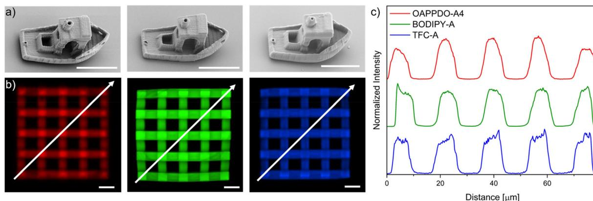
**Fig. 5** (a) The benchmarking structures consisting of boats were fabricated out of the same formulation as the lattice below and imaged *via* SEM (Scalebars = 10 μm). (b) 2PLP printed lattices with the red, green, and blue formulation, which were imaged *via* confocal microscopy. (c) The intensity of the respective lattice was plotted along the white arrow against the distance.
