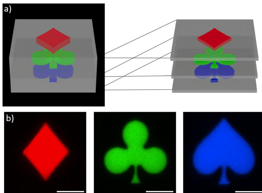
**Fig. 7** (a) Schematic figure of the z-stack multi-material print and the imaged planes are indicated *via* the three stacked images. (b) Single layer of the red, green, and blue part of the z-stack recorded *via* confocal microscopy (Scalebars = 5  $\mu\text{m}$ ).
