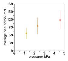
**Fig. 8** Results of peel tests when no activation of a 34.24 vol% PS in a PSA-latex film has occured, the average peel force is plotted as a function of pressure applied over a period of 7 days.
