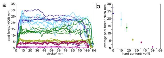
Fig. 5 90° peel testing of PS-PSA films, 2 cm in width, where the PS volume fraction (■ 0.00 vol%, ■ 10.15 vol%, 17.31 vol%, ■ 25.00 vol%, ■ 35.64 vol%, 50.10 vol%) in the dry state is varied. (a) The average force measured as a function of peel distance, stroke, for each repeat and (b) the average peel force calculated as a function of hard volume fraction in the PS-PSA film.
