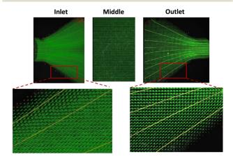
Fig. 2 Velocity vectors and streamlines at the inlet, middle section and outlet of the microfluidic chip for stimulated flow (13.125 mL h<sup>-1</sup>).
