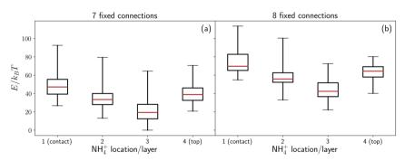
Fig. 5 Minimised energies of ammonium-containing ice for (a) seven and (b) eight (of a possible eight) fixed connections to the base. The whiskers show the extent of the energy range, with the box representing the first and third quartiles, and the red line showing the median. The energies have been shifted so that the minimum energy of all plotted configurations is 0. Any mechanically unstable structures have been removed.
