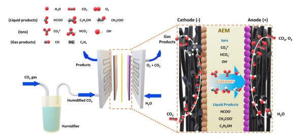
Fig. 1 Schematic overview of the crossover of the ions and liquid products in an MEA-type electrolyzer
