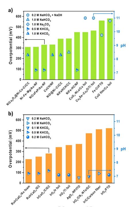
Performance and experimental conditions of (a) non-precious<sup>37-47</sup> and (b) precious<sup>48-53</sup> OER electrocatalysts in the aqueous carbonate system.
