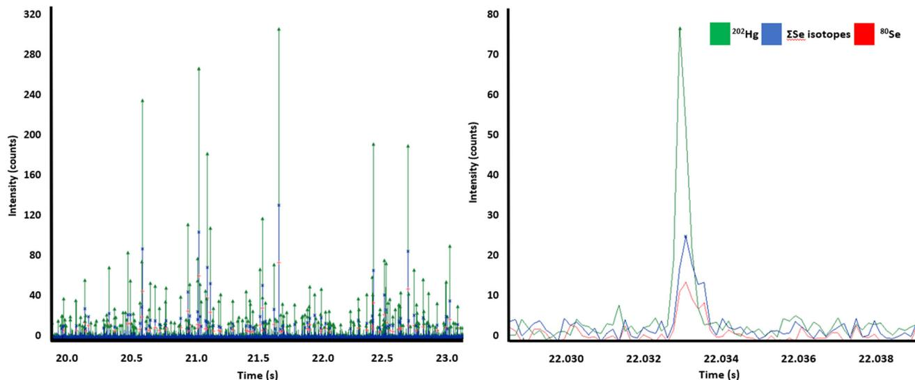
Fig. 3 The improvement of signal intensity when adding up all available isotopes of an element, like Se, is shown here. (Left) Hg/Se particles identified in a sperm whale liver sample. (Right) Shows the introduction of the sum of all Se isotopes, compared to the most abundant isotope ( $^{80}\text{Se}$ ). With this introduction comes the identification of a Hg/Se particle which would not have otherwise been identified as the signal for  $^{80}\text{Se}$  fell below the detection threshold.
