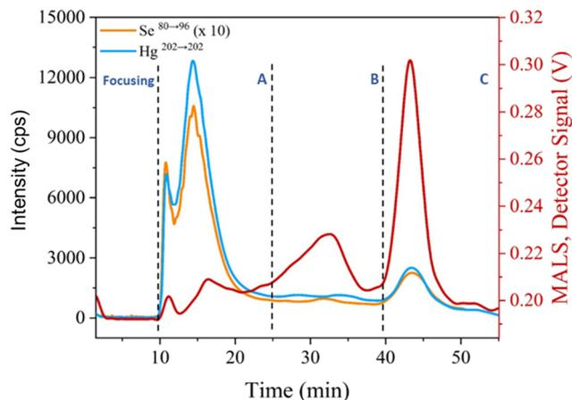
**Fig. 1** AF<sub>4</sub>-MALS-ICP-MS/MS analysis of a whale liver digest. The MALS signal is shown in red, while the blue and orange signals represent Hg and Se as detected by ICP-MS/MS. The figure is segmented into four sections by black dotted lines, the produced sections denote: focusing step, fraction A (10–25 minutes), fraction B (25–40 minutes), and fraction C (40–55 minutes).
