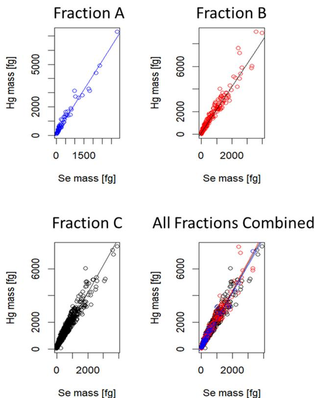
**Fig. 5** Shown are comparisons of the three slopes generated from plotting Hg mass vs. Se mass on particles which were separated by AF<sub>4</sub> and analysed by SP ICP-ToF-MS. The fourth plot shows all data combined with the three slopes also overlain, highlighting the similarity in the behaviour which is independent of particles size.
