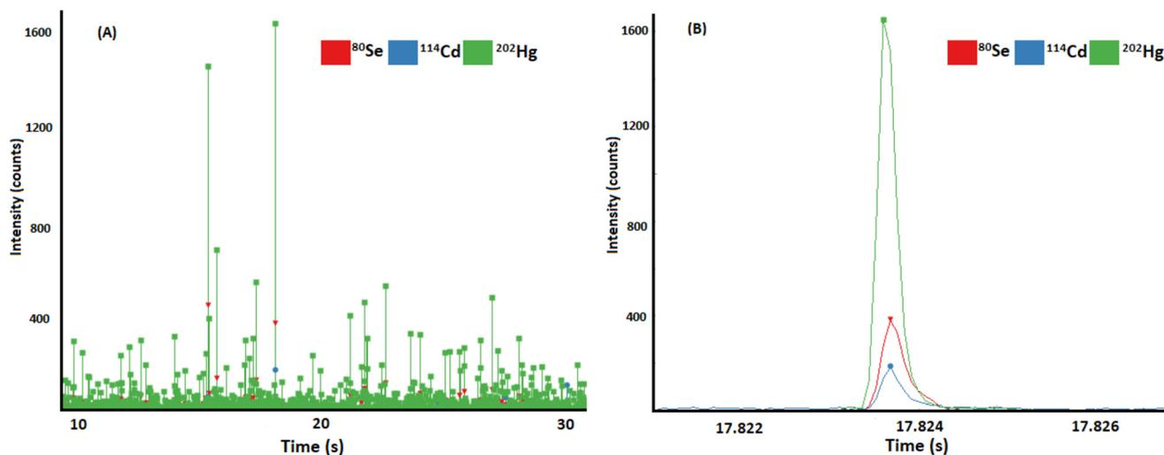
**Fig. 2** (A) Shows an example of the data produced from SP ICP-ToF-MS analysis of enzymatically digested sperm whale liver, where Hg, Se and Cd can be found. (B) Shows an example of a particle containing Hg, Se, and Cd.
