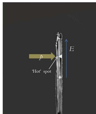
Fig. 4 Schematic presentation of the cracking of a growing column ice crystal (growth + cracking) under the influence of pressure ( $p$ ). The blue arrow represents an electric field  $E$ . The ‘Hot’ spot is a point at the tip of a crack with a highly localized electric field  $E_{\perp}^{\text{Cr}}$ .
