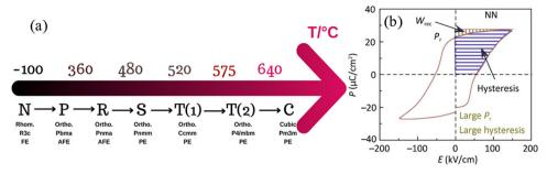
Fig. 6 (a) Phase transition of NN ceramics as a function of temperature (b) PE Loop of NN. 33 Reprinted (adapted) with permission from ref. 33 under the terms of the Creative Commons CC BY license, Elsevier.
