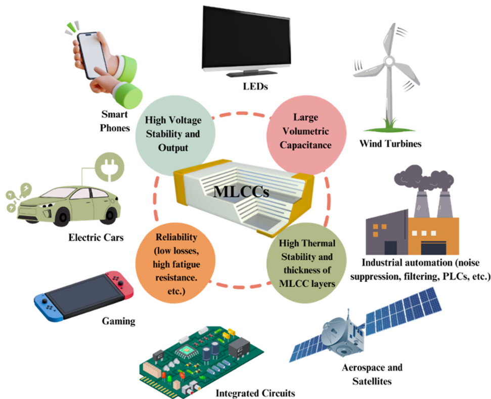
Fig. 3 Schematic diagram of MLCCs with key properties in developing the high energy performance and their different applications.
