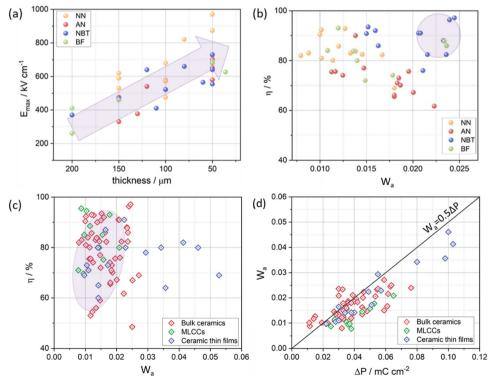
Fig. 19 Impact of thickness on (a)  $E_{\text{max}}$  (b) normalised  $W_{\text{a}} = W_{\text{rec}}/E_{\text{max}}$  and  $\eta$  in NN, AN, NBT, and BF-based ceramics (c) normalised  $W_{\text{a}}$  with  $\eta$  (d) normalised  $W_{\text{a}}$  with  $\Delta P$  in bulk ceramics, MLCCs, and thin films.
