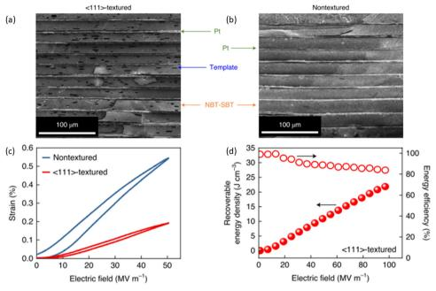
Fig. 24 SEM cross-section of (a) textured and (b) untextured NBT-SBT MLCCs. (c) S-E Loops of textured and nontextured MLCCs. (d) The energy storage performance of textured NBT-SBT MLCCs.<sup>205</sup> Reproduced from ref. 205 with permission from Springer Nature.
