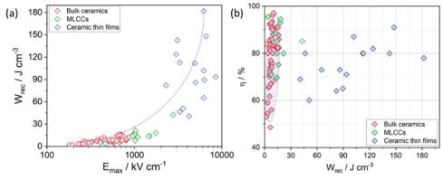
Fig. 18 The comparison between (a)  $E_{\text{max}}$  and  $W_{\text{rec}}$  and (b)  $W_{\text{rec}}$  and  $\eta$  in terms of thickness.
