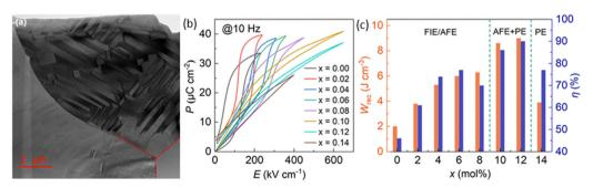
Fig. 8 (a) Overview of bright-field TEM image displaying three grains of the  $Ag_{0.64}Bi_{0.12}NbO_3 + 0.10$  wt%  $MnO_2$  ceramic (b) unipolar P-E loops measured at 10 Hz, and (c)  $W_{rec}$  and  $\eta$  of AN-xBi ceramics at room temperature. <sup>77</sup> Reproduced from ref. 77 with permission from the Royal Society of Chemistry.
