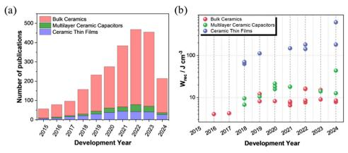
Fig. 2 (a) Number of publications, Web of Science (keywords of high energy density ceramics, multilayer ceramic capacitors, and ceramic thin films, excluding glass, polymer, and composite). (b) Development of  $W_{\text{rec}}$  in bulk ceramics, ceramic multilayers, and ceramic thin films for energy storage applications from 2015 to 2024.
