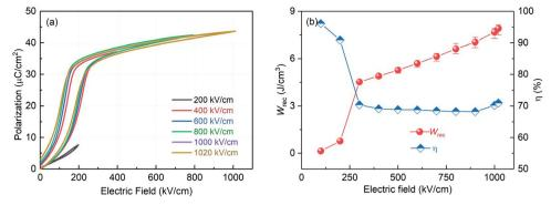
Fig. 15 Energy storage of ANT + Mn multilayer capacitors. (a) Unipolar P-E loops and (b)  $W_{\rm rec}$  and  $\eta$  measured at different electric fields from 200 kV cm<sup>-1</sup> to 1020 kV cm<sup>-1</sup>.81 Reproduced from ref. 81 with permission from the Royal Society of Chemistry.
