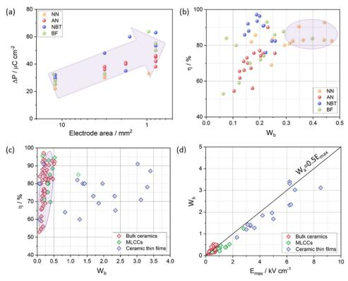
Fig. 20 The relationship between (a) electrode area and  $\Delta P$  in NN, AN, NBT, and BF-based ceramics (b) normalised  $W_b$  and  $\eta$  in NN, AN, NBT, and BFbased ceramics (c) normalised  $W_b$  and  $\eta$  in bulk ceramics, MLCCs, and thin films (d) normalised  $W_b$  and  $E_{max}$  in bulk ceramics, MLCCs, and thin films.
