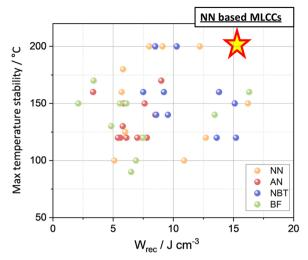
Fig. 26 Correlation between max temperature stability and  $W_{\rm rec}$  among four lead-free dielectric candidates.
