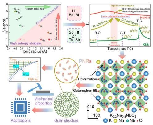
Fig. 23 Schematic overview of high-entropy design approach for KNN-based ceramics.<sup>240</sup> Reprinted (adapted) with permission from ref. 240 under the terms of the Creative Commons CC BY license, Springer Nature.
