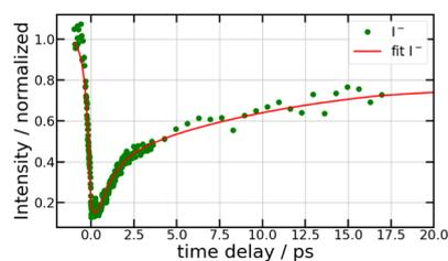
**Fig. 4 269/807 nm experiment** – Sum of the  $S_0^{\text{anion}}(\text{KER}, \tau)$  fs-TRKERS for anion energies between 0.09 and 0.17 eV as a function of the pump-probe delay (green dots). The full red curve best fits the experimental signal as described in the text, using the time constants  $\tau^-$ ,  $\tau_A$  and  $\tau_B$  listed in Table 1.
