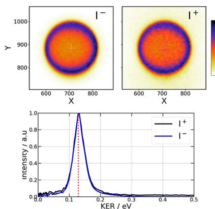
**Fig. 2 Pump only experiment at 269 nm** – Raw VMI images of  $I^-$  (top left panel) and  $I^+$  (top right panel) and kinetic energy release (KER) (bottom panel) for each ion. The red dashed line in the bottom panel is the expected KER energy from energy conservation. The colour scale for intensities in the  $I^-$  and  $I^+$  images is shown at the right hand side of the figure.
