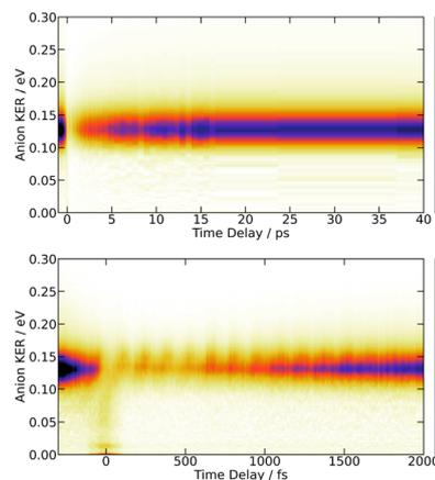
**Fig. 3 269/807 nm experiment** – 3D-plot of the fs-TRKERS signal  $S_0^{\text{anion}}(\text{KER}, \tau)$ , up to 40 ps (top panel) and 2 ps (bottom panel): the signal intensity is given by the colour map shown at the right hand side of the figure; it is plotted as a function of the  $I^-$  KER energy (vertical axis in eV) and pump-probe delay (horizontal axis).
