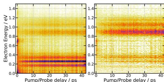
Fig. 7 269/807 nm experiment – 3D-plot of the fs-TRPES signals  $S_0^{\text{elec}}(E,\tau)$  (left panel, isotropically distributed photoelectrons) and  $S_2^{\text{elec}}(E,\tau)$  (right panel, polarised electrons) with the same colour map as in Fig. 3.
