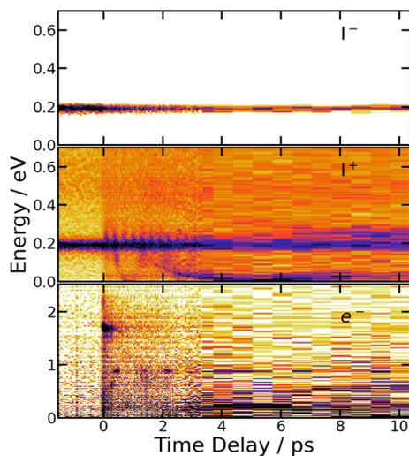
Fig. 9 266/334 nm experiment – 3D-picture of  $S_0^{\text{elec}}(E, \tau)$  (bottom panel),  $S_0^{\text{cation}}(E, \tau)$  (middle panel) and  $S_0^{\text{anion}}(E, \tau)$  (top panel) using the same colour map as in Fig. 3.
