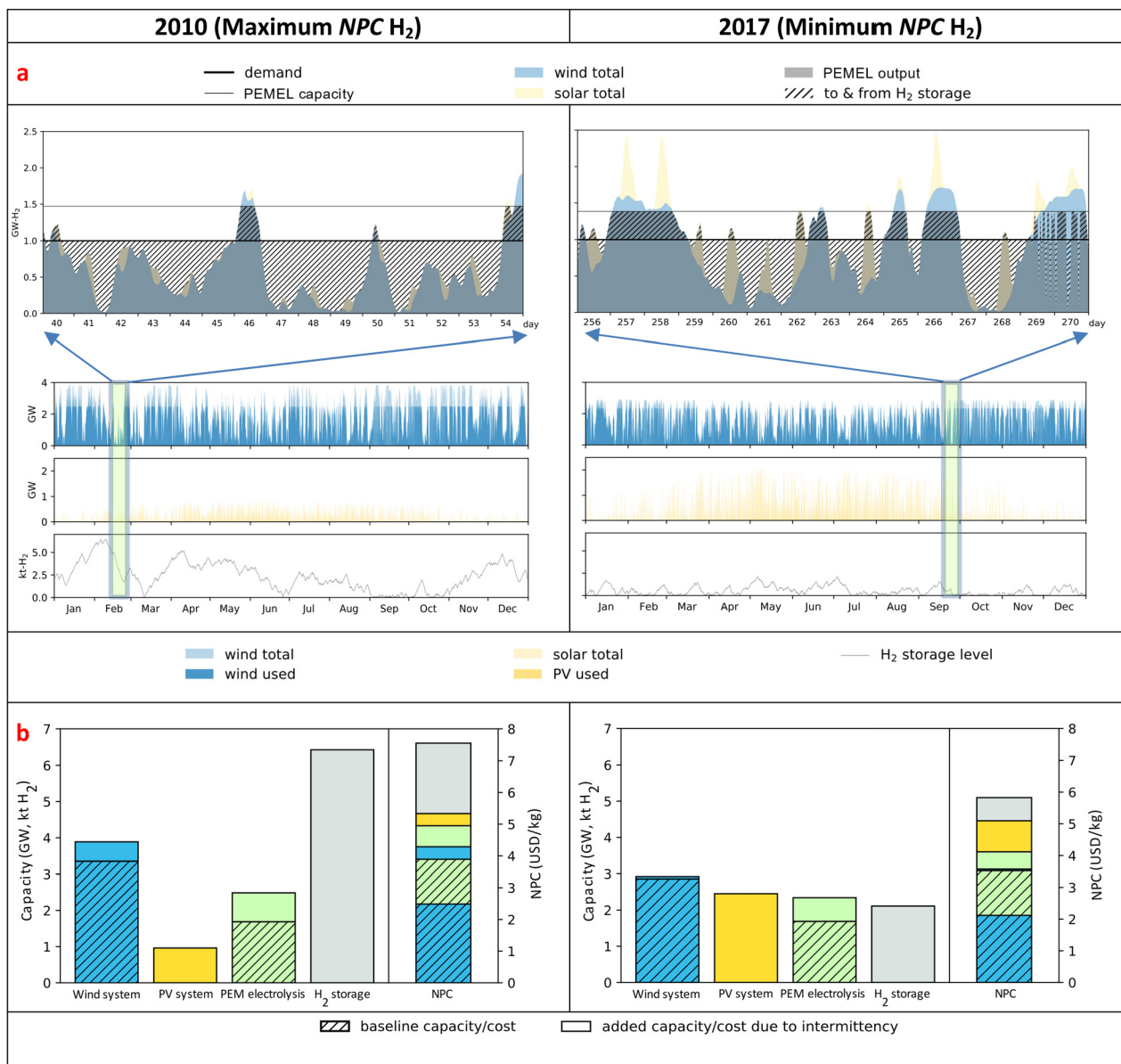
Fig. 9 Energy profiles and cost of the system, including the “cost of intermittency” for the year with maximum (2010) and minimum (2017) NPC of green H 2 for the Isle of Jura in the UK. The solar and wind profiles of the total available energy and energy used are shown in subplot a, along with the H 2 storage levels for the system producing a continuous flow of H 2 (1 GW) without considering the sale of surplus electricity. The capacity of the system components and their NPC, including the cost due to intermittency, are shown in subplot b. The cost of intermittency represents ca. 49% and 41% of the total production cost of green H 2 for 2010 and 2017, respectively.
