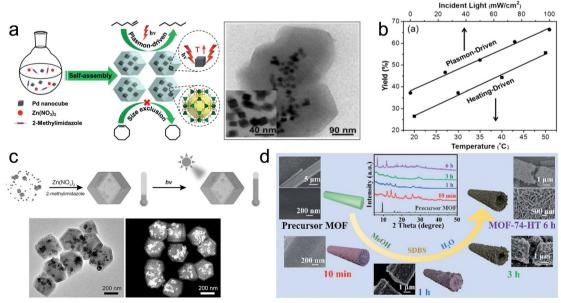
Fig. 7 (a) Self-assembly of Pd NCs@ZIF-8 and plasmon-driven selective catalysis of hydrogenation of olefins. (b) The hydrogenation performance of Pd NCs@ZIF-8.<sup>69</sup> (c) Schematic illustration of the formation of Au&Pt@ZIF and temperature variation under light irradiation.<sup>70</sup> (d) Phase transformation from the MOF precursor to MOF-74-HT.71
