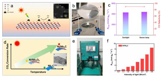
Fig. 6 (a) Schematic illustration and TEM image of the  $Ru/Mo_2TiC_2$  photothermal catalyst. (b) Setup of the outdoor photothermal catalysis. (c)  $CO_2$  conversion and product selectivity of  $Ru/Mo_2TiC_2$  in photothermal catalytic RWGS.<sup>68</sup> (d) Schematic illustration and TEM image of the Ni/Ni<sub>2</sub>C photothermal catalyst. (e) Photograph of the batch reactor. (f) Photothermal catalytic activity of Ni/Nb<sub>2</sub>C in photothermal catalytic RWGS.<sup>28</sup>
